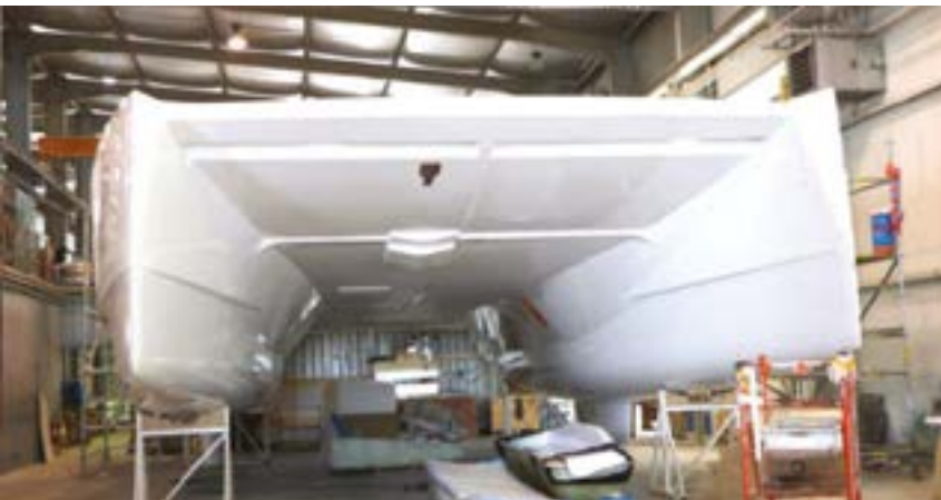
One-piece deck and hulls for increased structural rigidity
