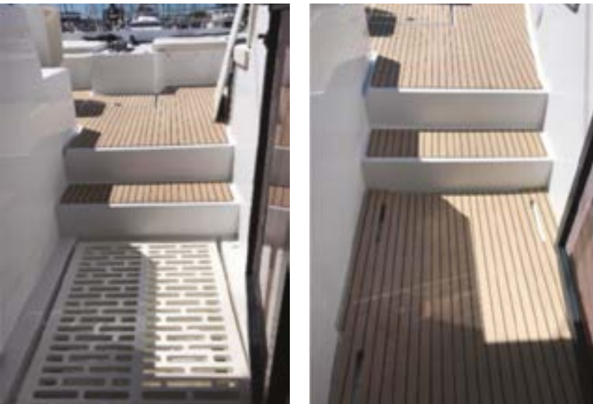
Grating open during navigation and closed for mooring
